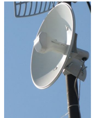
Fig. 10. The client station of a communication network of NSSM for long distances
