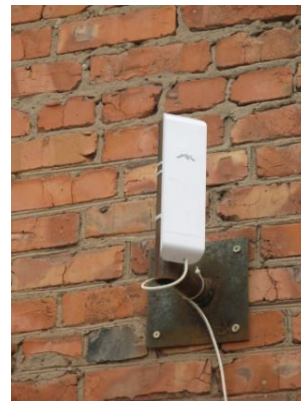
Fig. 9. The client station of a communication network of NSSM for average distances
