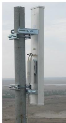
Fig. 8. Access point of the center of a wireless communication network of NSSM
