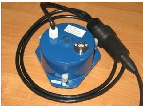
Fig. 4. NSSM geophone for the surface installation
