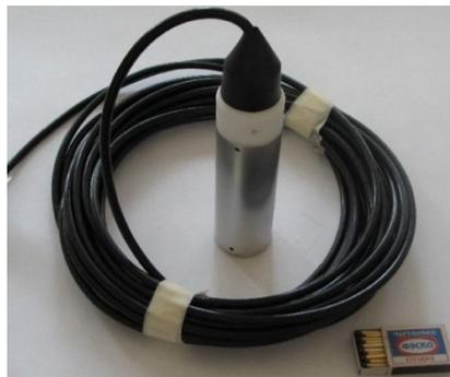
Fig. 5. A geophone for well installation
