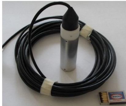
Fig. 5. A geophone for well installation
