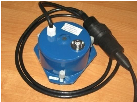
Fig. 4. NSSM geophone for the surface installation
