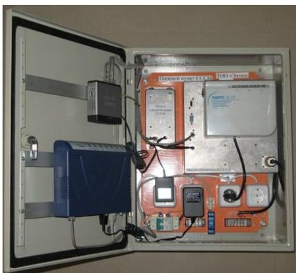
Fig. 7. Field unit of the NSSM system for underground installation
