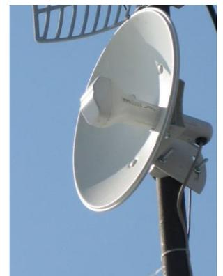
Fig. 10. The client station of a communication network of NSSM for long distances
