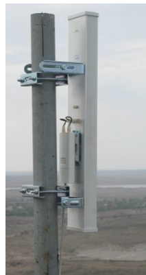
Fig. 8. Access point of the center of a wireless communication network of NSSM
