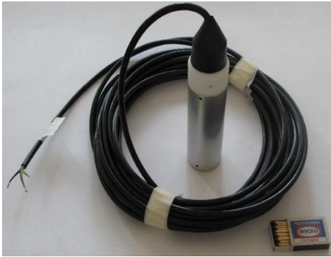
Fig. 7. The geophone for well installation
