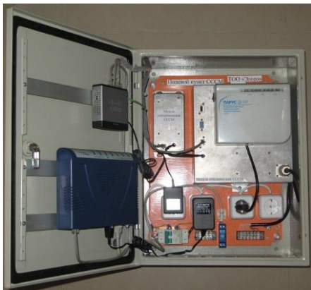
Fig. 9. Field unit of the NSSM system for underground installation
